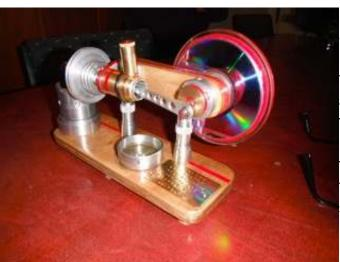
Ken McIntyre had his #3 horizontal Stirling hot-air engine operating. He has been having problems with a smaller version of the engine in getting it going and suspects the piston size is too small for capacity and correct heat transfer. He has been using old CD discs in the flywheels for visual effect and showed the jig he used for machining discs to size. These discs are laminated and need careful cutting from both faces to prevent breakage. Tom Hood has
