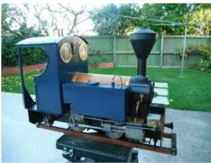
Nigel Wood has been making a spark arrestor for his Sweet Pea after getting cinder burns. Making the base collar for the chimney from a brass billet has been interesting. A plug was cut from the centre of the billet by water jet to save a large pile of expensive swarf in the machining process and the collar just needs to have the radiused section finished off. It remains to be seen how effective the new chimney will
